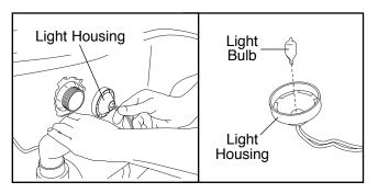
To replace the light bulb, pull the old light bulb out of the housing and insert a new light bulb. Re-attach the light housing to the spa shell. Re-attach the access panel to the spa.
